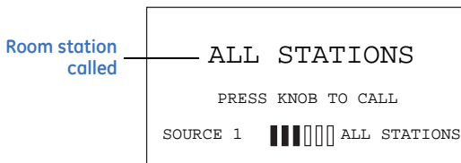
Figure 4. Intercom control screen
