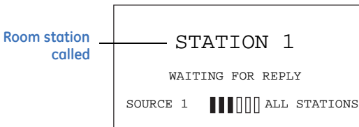
Figure 7. Calling room station Intercom screen
